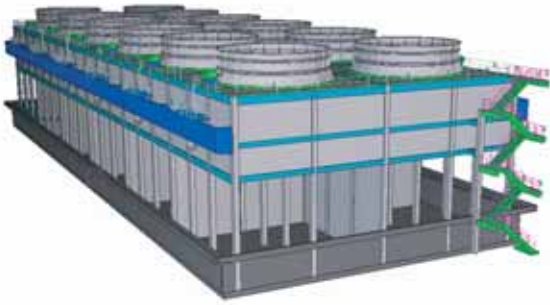
:: Bang Pakong Power Plant Thailand, 35800 m 3 /hr (12-cell back to back).
